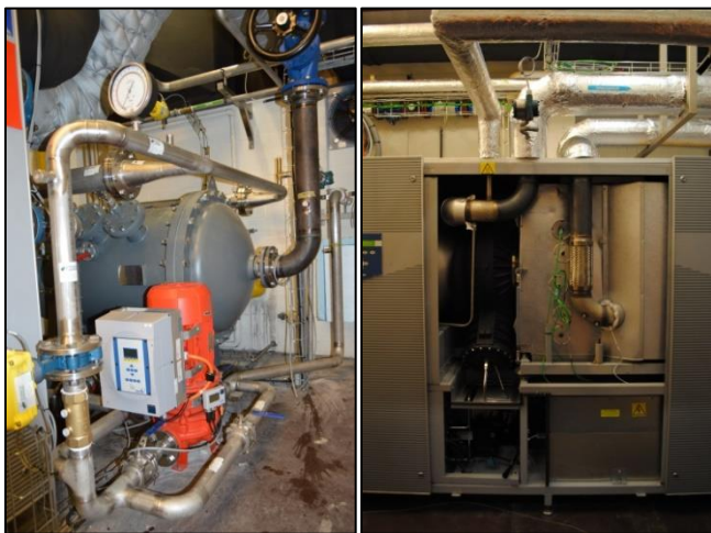
Figure 2. Saturator for VUB-mHAT system (left), T100 test rig modified to connect with humidification unit (right).
